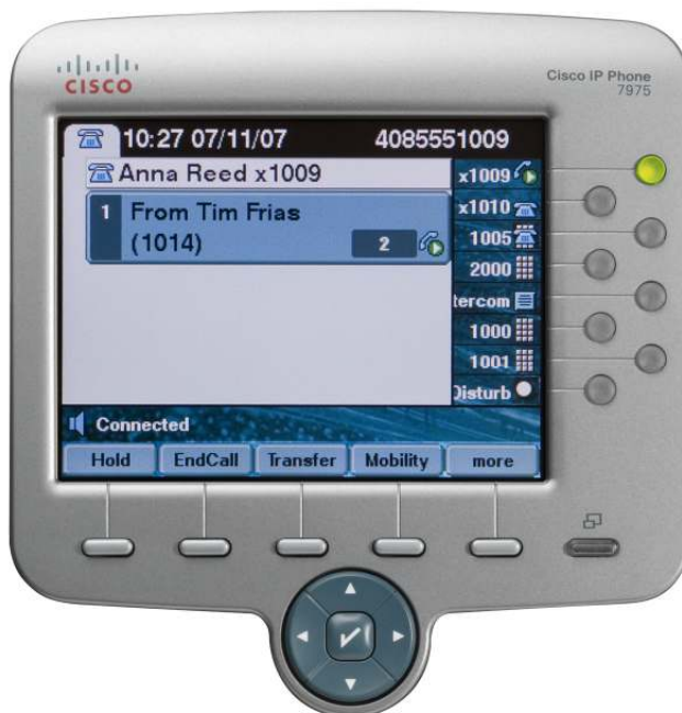
Figure 2. Close-Up of Display and Lighted Line Keys
